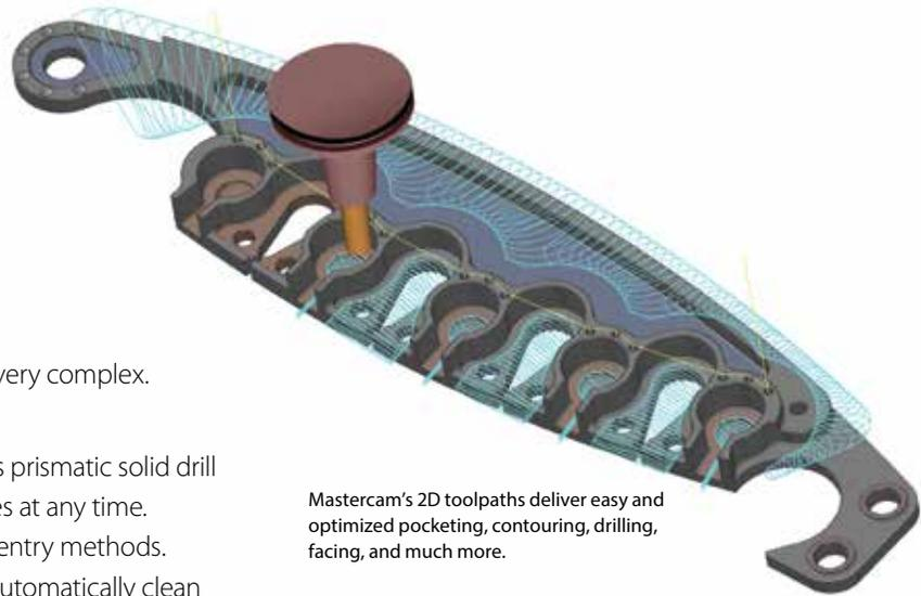
Mastercam's 2D toolpaths deliver easy and optimized pocketing, contouring, drilling, facing, and much more.
